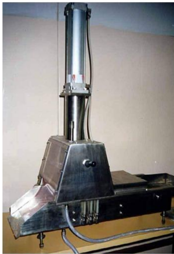
Fig. 2. Automatic brine injector Ya5-FSh1L of two pneumatic drives
