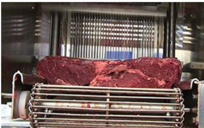
Fig. 1. Beef being mechanically tenderized by blades [15]
