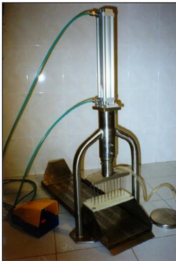
Fig. 1. Ya5-FShM brine injector with manual feed of raw materials and pneumatic drive of brine supply and needle block lowering
